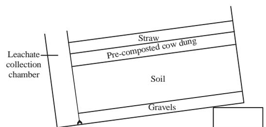
Fig. 2: Illustration of vermicomposting leachate reactor setup
