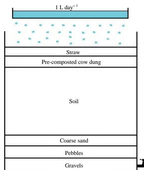
Fig. 1: Illustration of vermiwash reactor setup
